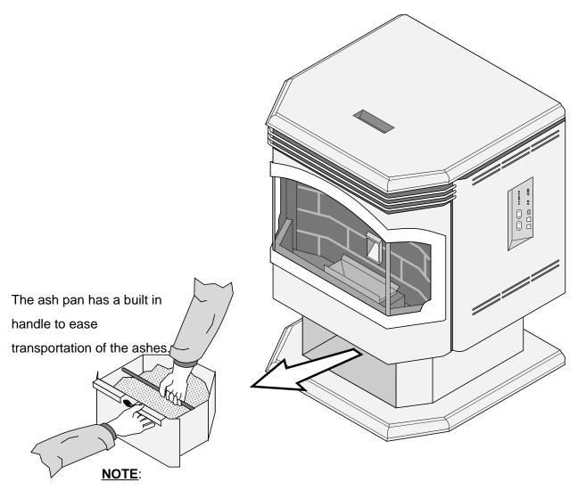
When replacing the ash pan make sure it is pushed all the way in.
